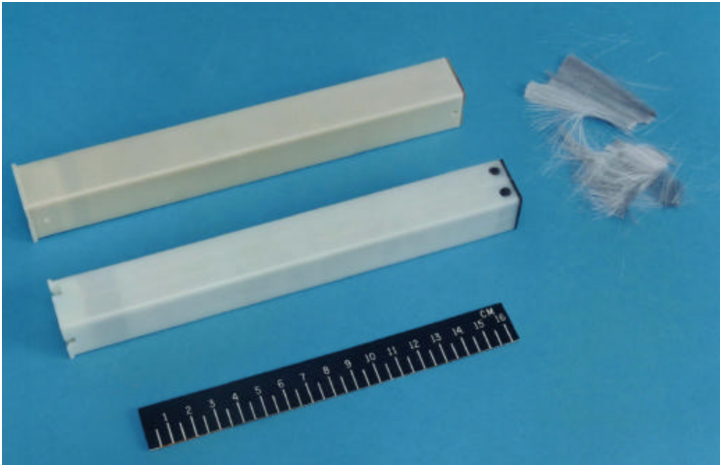
Training and operation RF chaff rounds used by the USAF. RR-188 (top) and RR-180 (bottom).
