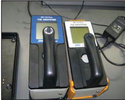
Figure 1-8. GR-135 IdentifINDER. The IdentifINDER is automatically in the search and data mode. It displays simultaneously. Should high levels of radiation be detected, the unit gives an eyes-free audio alert to the operator to the location of the source. If radiation levels are high, the unit tells the operator to back off.
