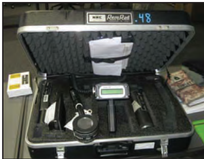
Figure 1-9. The ADM-300, an all-in-one multifunctional detection system for rapid response to suspected radiation hazards. ADM-300s are rugged, reliable, and designed for use in harsh environments. The ADM-300 will detect, measure, and digitally display both dose and dose rate levels of radiation from 10 \mu\text{R/hr} to 10,000 R/hr and beta audio alert and aids in directing radiation from 10 \mu\text{R/hr} to 5 R/hr (0.1 \mu\text{Sv/hr} to 0.05 Sv/hr).
