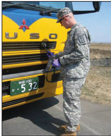
Figure 1-10. A 71st Chemical Company Soldier using the ADM-300 to detect and measure radiation
