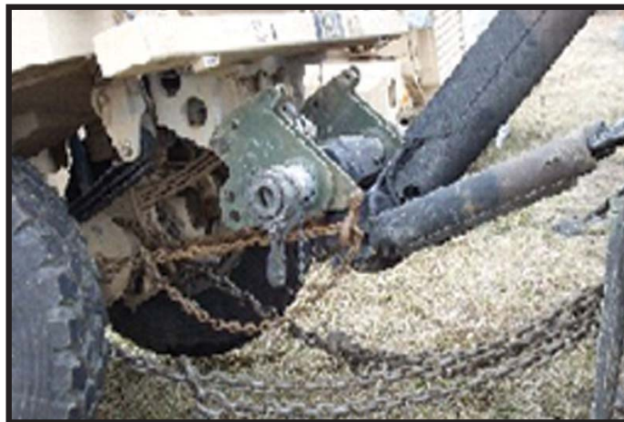
Figure A-25: HEMTT/MTVR wrecker front lift tow with MUAs (NSN 5340-01-516-2058 [L] and NSN 5340-01-516-2059 [R])
