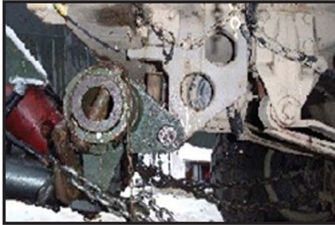
Figure A-24: HEMTT/MTVR wrecker front lift tow with HEMTT BII adapter D (NSN 2590-01-226-3349 [L] and NSN 2540-01-226-7139 [R])
