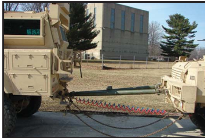
Figure A-41: GDLS connected to a U.S. Army heavy duty tow bar
