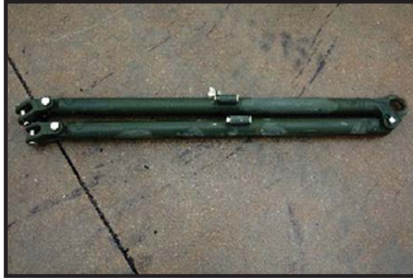
Figure A-46: U.S. Army heavy duty tow bar (NSN 2540-01-267-2912)
