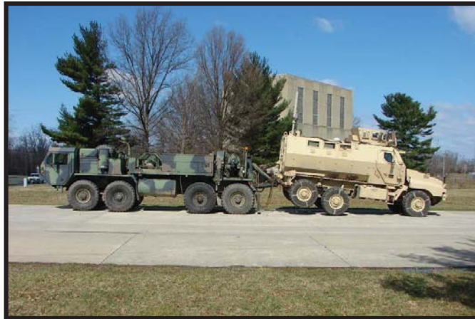
Figure A-17: HEMTT/MTVR wrecker rear lift tow with MUAs (NSN 5340-01-516-2058 [L] and NSN 5340-01-516-2059 [R])
