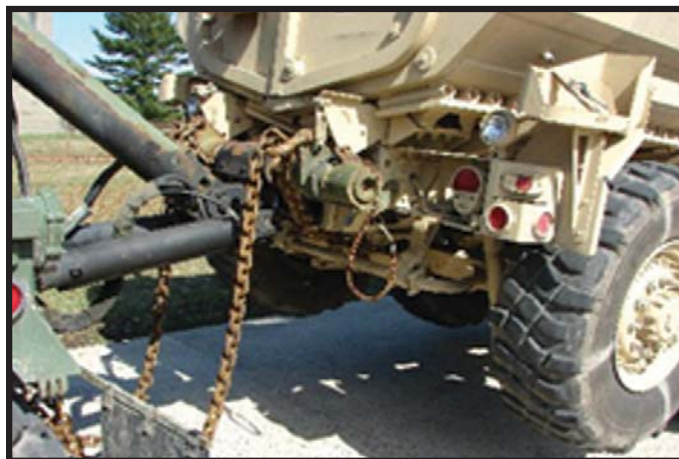
Figure A-18: HEMTT/MTVR wrecker rear lift tow with HEMTT BII adapter F (NSN 2590-01-226-3351 [L] and NSN 2540-01-226-3350 [R])
