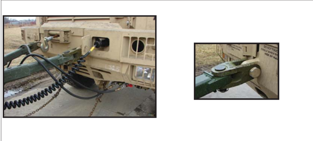
Figure A-40: USMC MTRV tow bar (NSN 2350-01-496-8356) and adapter (NSN 2540-01-500-5325) and shackle pin
