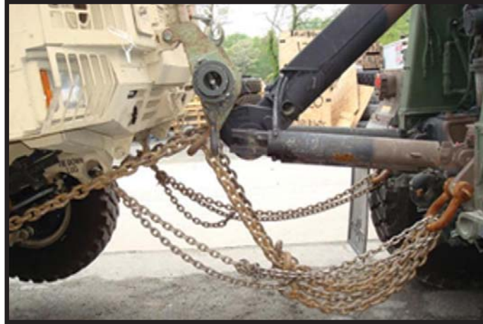
Figure A-43: HEMTT/MTVR wrecker front lift tow with HEMTT BII adapter D or F (NSN 2590-01-226-3349 [L] and NSN 2540-01-226-7139 [R])
