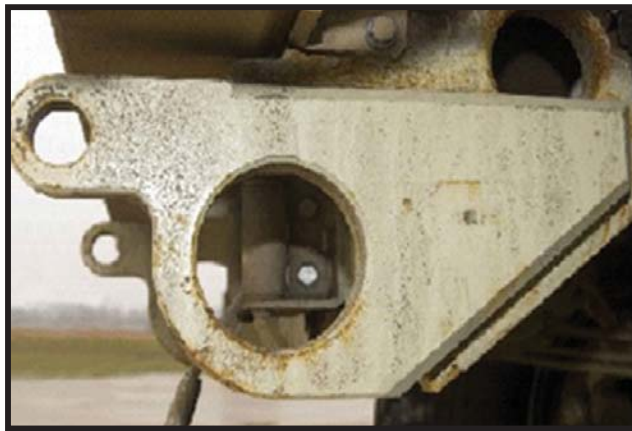
Figure A-23: Cougar modified front tow lug, 1.5 in. thick lug and 1.5 in. pin diameter
