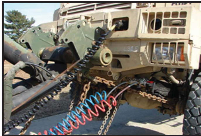
Figure A-44: HEMTT/MTVR wrecker front lift tow with MUAs (NSN 5340-01-516-2058 [L] and NSN 5340-01-516-2059 [R])
