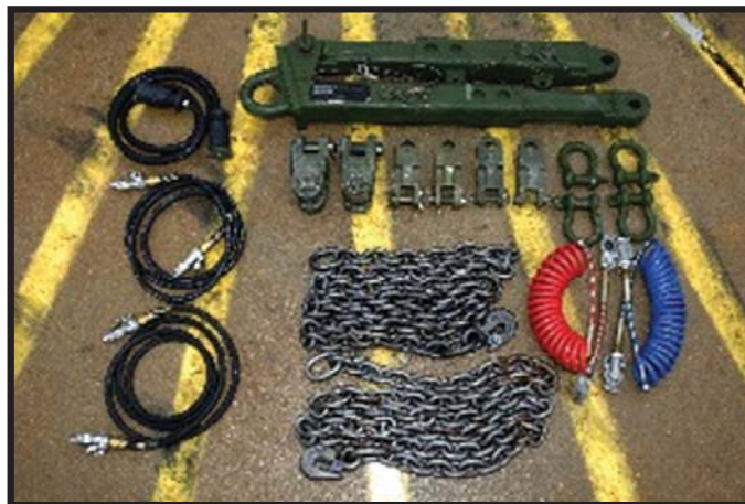
Figure A-45: USMC MTVR tow bar kit (NSN 2350-01-496-8356)
