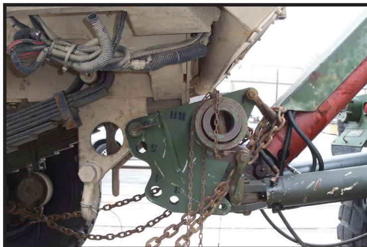
Figure A-7: HEMTT/MTVR wrecker front lift tow with MUAs (NSN 5340-01-516-2058 [L] and NSN 5340-01-516-2059 [R])
