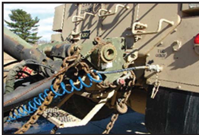
Figure A-26: HEMTT/MTVR wrecker rear lift tow with MUAs (NSN 5340-01-516-2058 [L] and NSN 5340-01-516-2059 [R])
