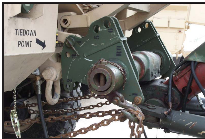
Figure A-8: HEMTT/MTVR wrecker rear lift tow with MUAs (NSN 5340-01-516-2058 [L] and NSN 5340-01-516-2059 [R])
