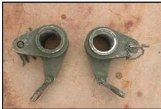
Figure A-36: HEMTT wrecker BII adapter D (NSN 2590-01-226-3349 [L] and NSN 2540-01-226-7139 [R])
