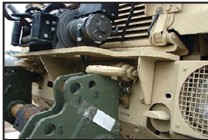
Figure A-16: HEMTT/MTVR wrecker front lift tow with MUAs (NSN 5340-01-516-2058 [L] and NSN 5340-01-516-2059 [R])
