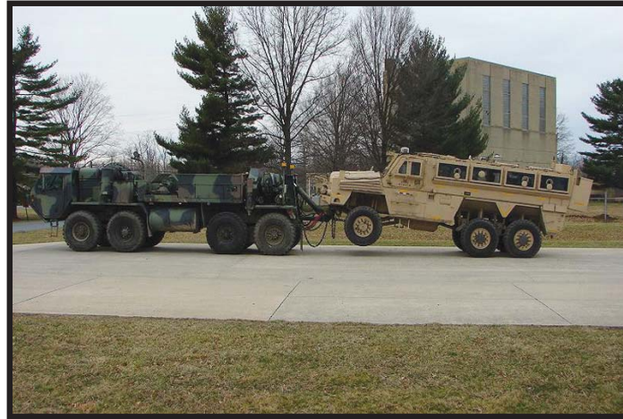
Figure A-5: Heavy expanded mobility tactical truck (HEMTT) wrecker lift towing BAE 6X6
