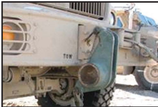
Figure A-33: HEMTT wrecker BII adapter F (NSN 2590-01-226-3351 [L] and NSN 2590-01-226-3350 [R])
