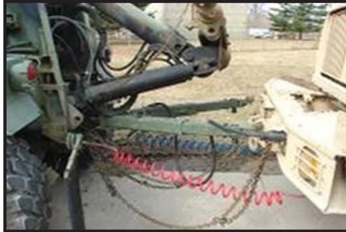
Figure A-31: HEMTT wrecker flat towing IMG MaxxPro with USMC MTRV towbar
