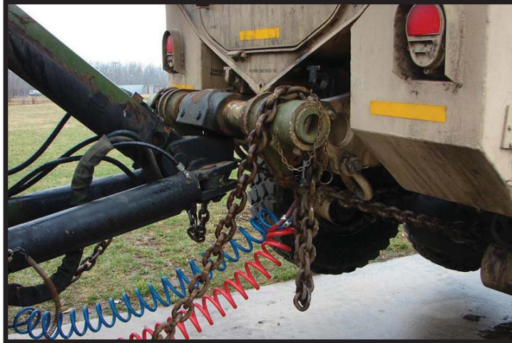
Figure A-9: HEMTT/MTVR wrecker rear lift tow with HEMTT BII adapter D (NSN 2590-01-226-3349 [L] and NSN 2540-01-226-7139 [R])
