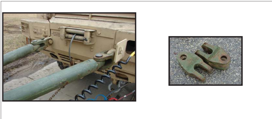
Figure A-39: U.S. Army heavy duty tow bar (NSN 2540-01-267-2912) and adapter (NSN 5340-01-267-2908) and shackle pin
