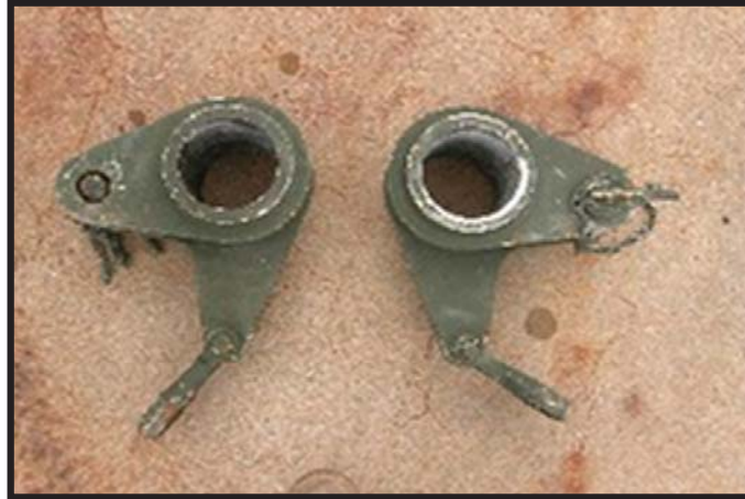
Figure A-27: HEMTT wrecker BII adapter D (NSN 2590-01-226-3349 [L] and NSN 2540-01-226-7139 [R])
