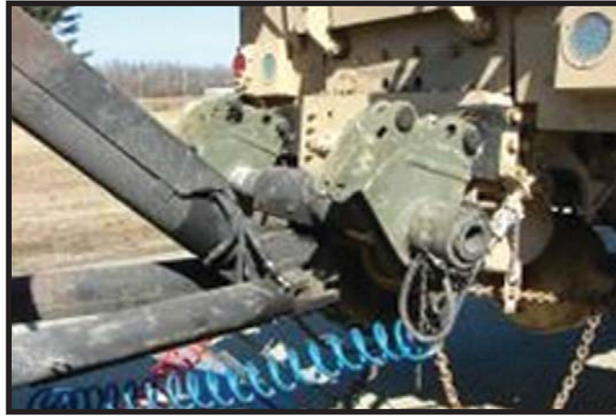
Figure A-35: HEMTT/MTVR wrecker rear lift tow with MUAs (NSN 5340-01-516-2058 [L] and NSN 5340-01-516-2059 [R])
