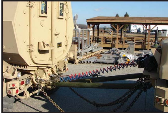
Figure A-13: BAE-TVS Caiman connected to a U.S. Army heavy duty towbar
