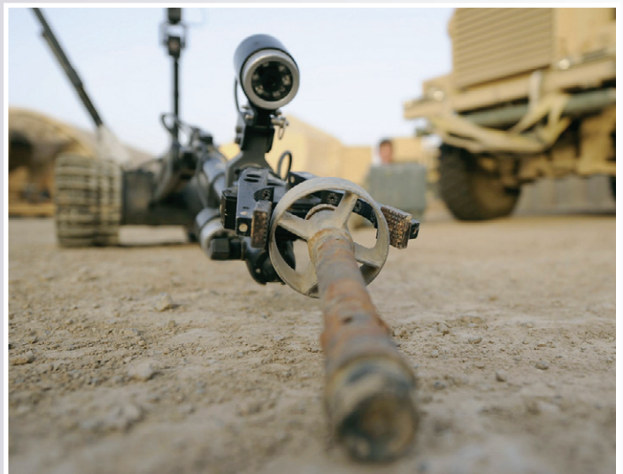
The arm of a Talon robot grasps a mortar tail during an operations check on the robot at Forward Operating Base, Azizullah, Afghanistan. The robot is used to interrogate IEDs when explosive ordnance disposal personnel need to investigate an IED from a safe distance. (Photo by Staff Sgt. Stephen Schester)
