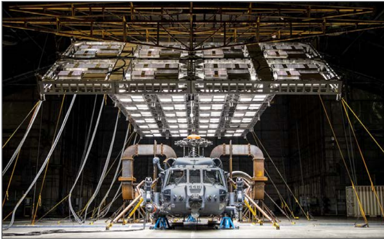
An HH-60W Jolly Green II sits under bright lights used to create heat in the McKinley Climatic Lab at Eglin Air Force Base.
