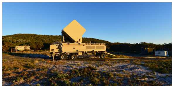
REPROGRAMMABLE GROUND-BASED RADAR SIGNAL EMULATOR FOR USE IN OPEN-AIR TESTING OF ADVANCED AIR PLATFORMS, INCLUDING THE JOINT STRIKE FIGHTER
