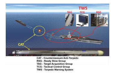
The operator uses these displays to manage the threat engagement sequence and command CAT launches.
