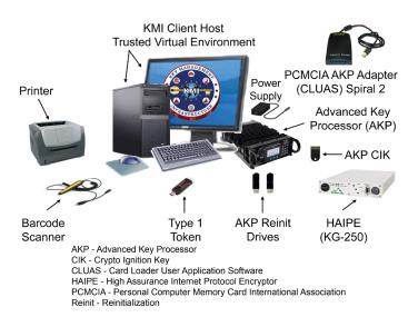
• KMI combines substantial custom software and hardware development with commercial off-the-shelf computer components. The custom hardware includes an Advanced Key Processor for autonomous cryptographic key generation and a Type 1 user token for role-based user authentication. The commercial off-the-shelf components include a client host computer with monitor and peripherals, High Assurance Internet Protocol Encryptor (KG-250), printer, and barcode scanner.
