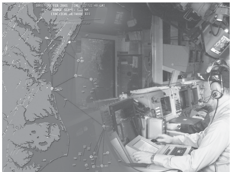
The Cooperative Engagement Capability is a system of hardware and software that allows ships to share radar data on air targets.
