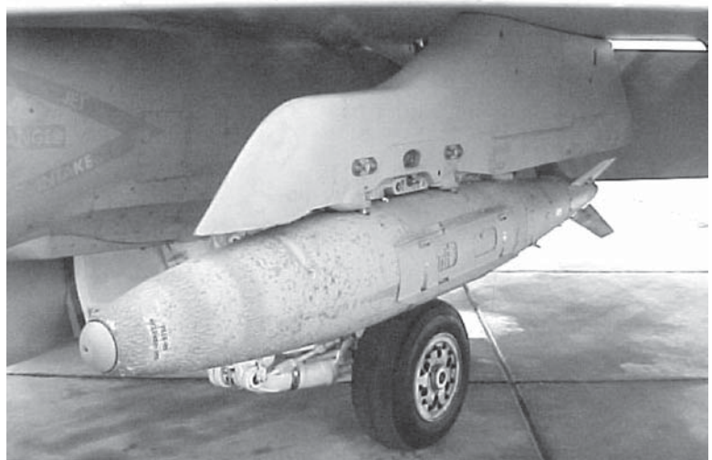
MOT&E of the 1,000-pound JDAM variant delivered during the F/A-18 phase of operational testing confirmed operational effectiveness and suitability of the 1,000-pound Joint Direct Attack Munition when delivered from this aircraft.
