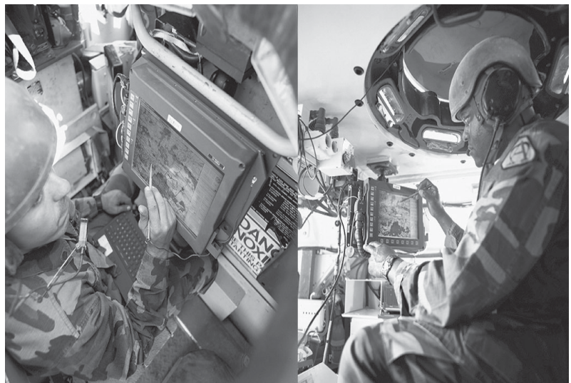
The Force XXI Battle Command, Brigade and Below is a digital battle command system that provides information to support a brigade task force.
