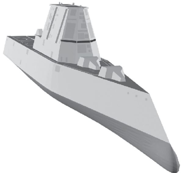
DD(X) will be a multi-mission destroyer featuring a composite deckhouse and a Wave-Piercing Tumblehome Hull displacing about 14,000 tons.
