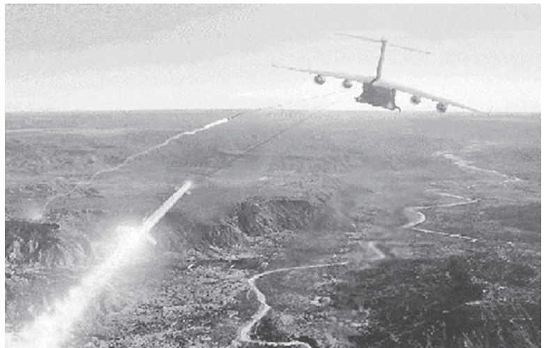
The Large Aircraft Infrared Countermeasures system is to provide protection against man-portable, shoulder-fired, and vehicle-launched infrared guided missiles.
