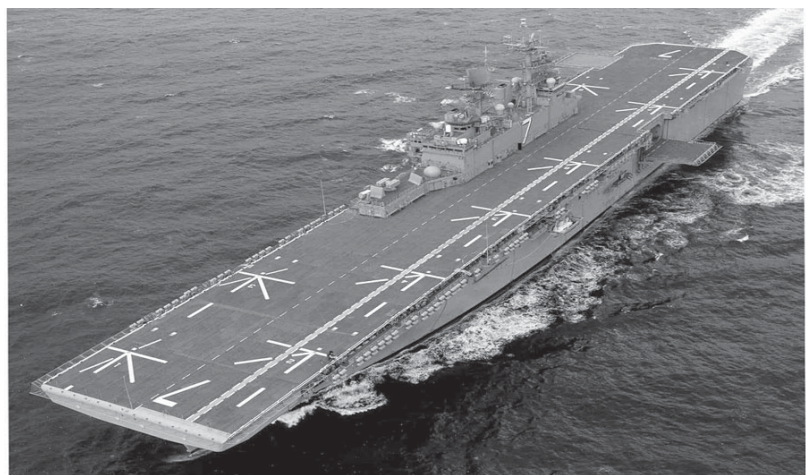
Although labeled as the last of the USS Wasp (LHD 1-7) class ships, there are important differences in LHD 8. The most significant change is to the propulsion system, in which the previous steam system is replaced with gas turbines, a machinery control system, and auxiliary propulsion motors.
