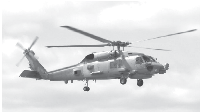
The MH-60R combines the missions of the legacy SH-60B and SH-60F aircraft into a single airframe.
