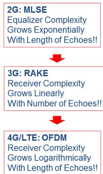
**Figure 1.3:** 2G, 3G, 4G Receiver Complexity
