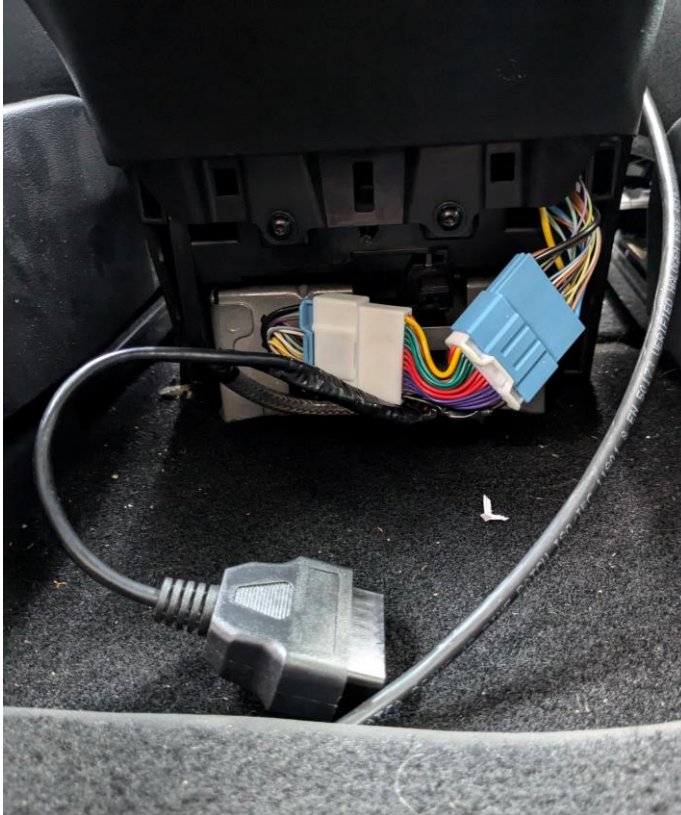
CAN adapter installed in the middle console of a Tesla Model 3
