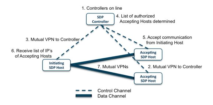
Figure 2: Workflow of the architecture of the Software Defined Perimeter
