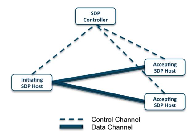
Figure 1: The architecture of the Software Defined Perimeter consists of two components: SDP Hosts and SDP Controllers
