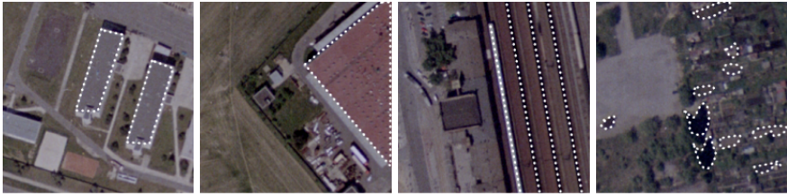
Fig. 2. Various shapes detected in orthophoto maps - rectangles, triangles, lines and anomalies
