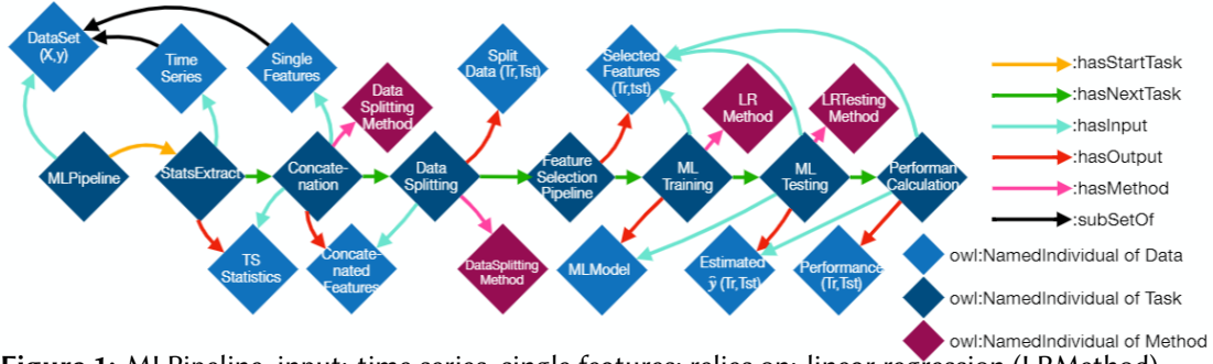
Figure 1: MLPipeline, input: time series, single features; relies on: linear regression (LRMethod).
