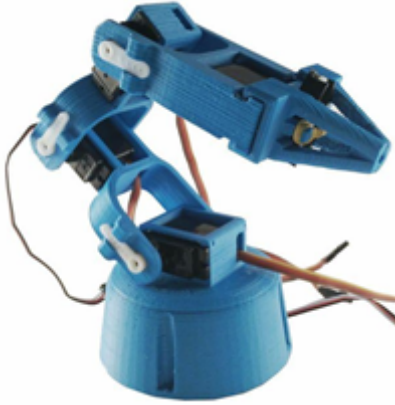
Figure 8: 3D printed robot arm based on Arduino robotic platform.
