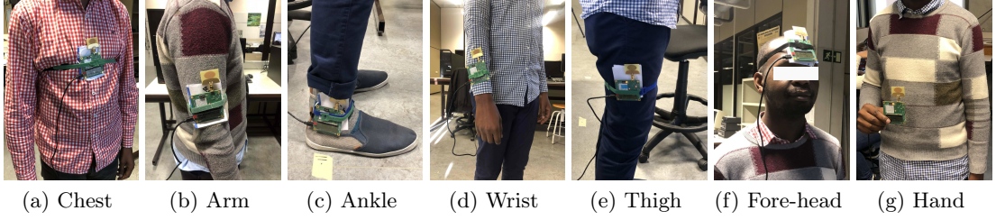
Fig. 2: Wearable sensors mounted at different positions on the body. At the hand, the sensor is about 20 cm from the chest since this is a usual place for texting or looking at the screen of a smart phone when locating your position in a real world scenario.
