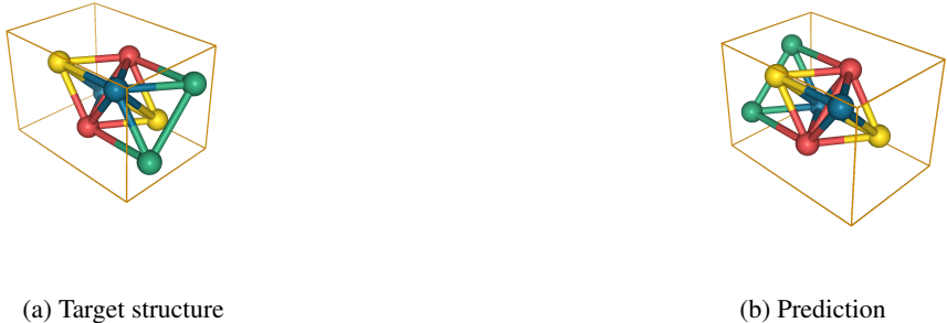
Figure 4: Example of using PBC-aware loss. The depicted structures ( \text{Mo}_2\text{Nb}_2\text{Ta}_2\text{W}_2 ) are visually different, but in fact they are exact the same. It is confirmed by insignificant value of PBC-aware loss
