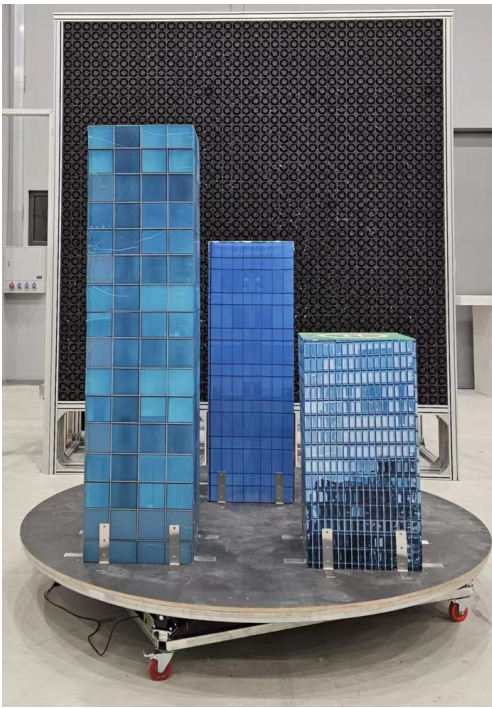
FIG. 19. Experimental configuration of the scaled building cluster configuration on a rotating ‘round dish’.
