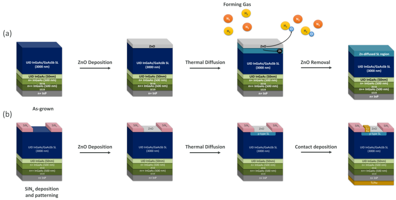
FIG. 1. (a) Schematic of the diffusion process using the as-grown sample and atomic layer deposition (b) Fabrication process for the planar Diodes
