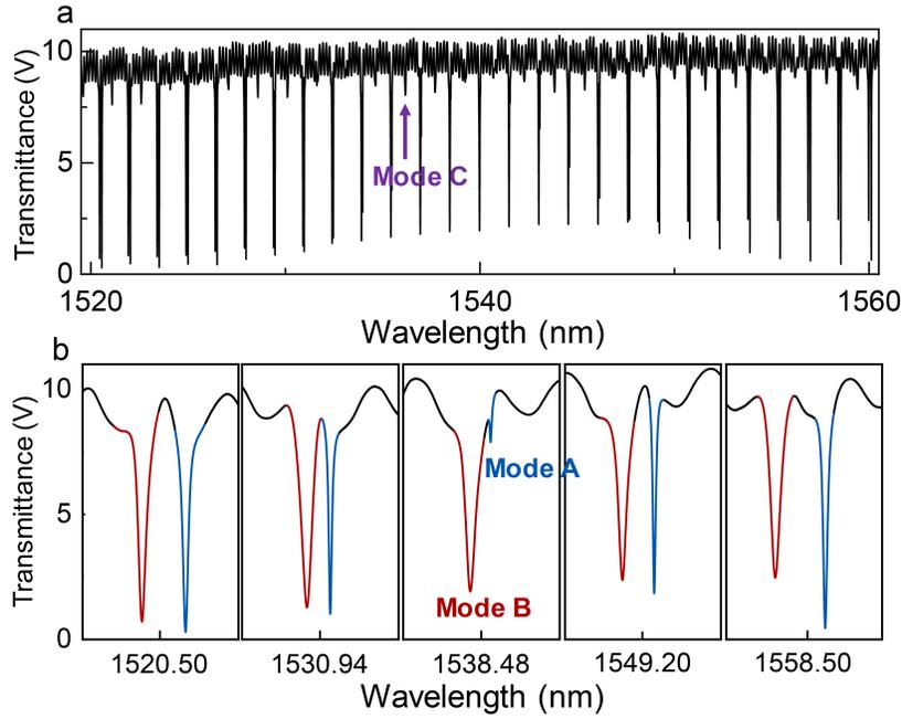
Fig. 3. Transmission spectrum near the avoided resonance crossing region. (a) Wide-range transmission spectrum of the Limaçon microdisk with  $\epsilon = 0.35$ . (b) Zoom-in view of spectra in (a) before, near, and after the strong coupling regions. Clear variations in resonant wavelength difference and resonant linewidths are observed. Each spectrum in (b) has a fixed wavelength range of 0.4 nm.
