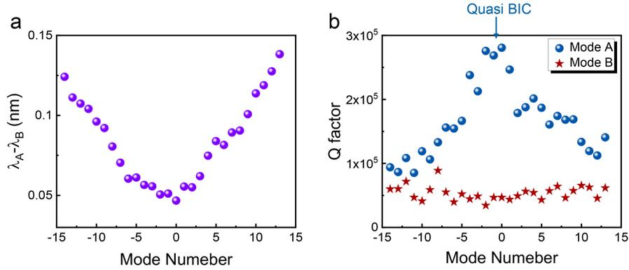
Fig. 4. Formation of Friedrich-Wintgen quasi-BIC. The resonant wavelength difference in (a) and  $Q$  factors of Mode A and Mode B in (b) are extracted from the spectrum in Fig. 2(a) by Lorentzian fitting. Mode number 0 corresponds to resonances at a wavelength of 1538.48 nm. Avoided resonance crossing along with the significantly enhanced  $Q$  factor of Mode A indicates the formation of Friedrich-Wintgen quasi-BIC.
