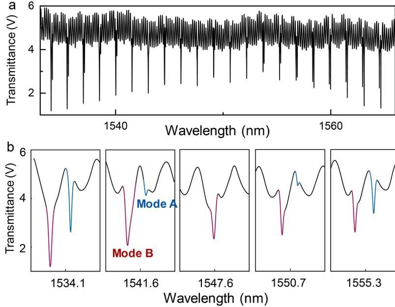
Fig. 6. Formation of Friedrich-Wintgen quasi-BIC in a single Limaçon microcavity with  $\epsilon = 0.4$ . (a) Wide-range transmission spectrum of the Limaçon microcavity with  $\epsilon = 0.4$ . (b) Zoom-in view of spectra in (a) before, near, and at strong coupling. Each spectrum has a fixed wavelength range of 0.4 nm.
