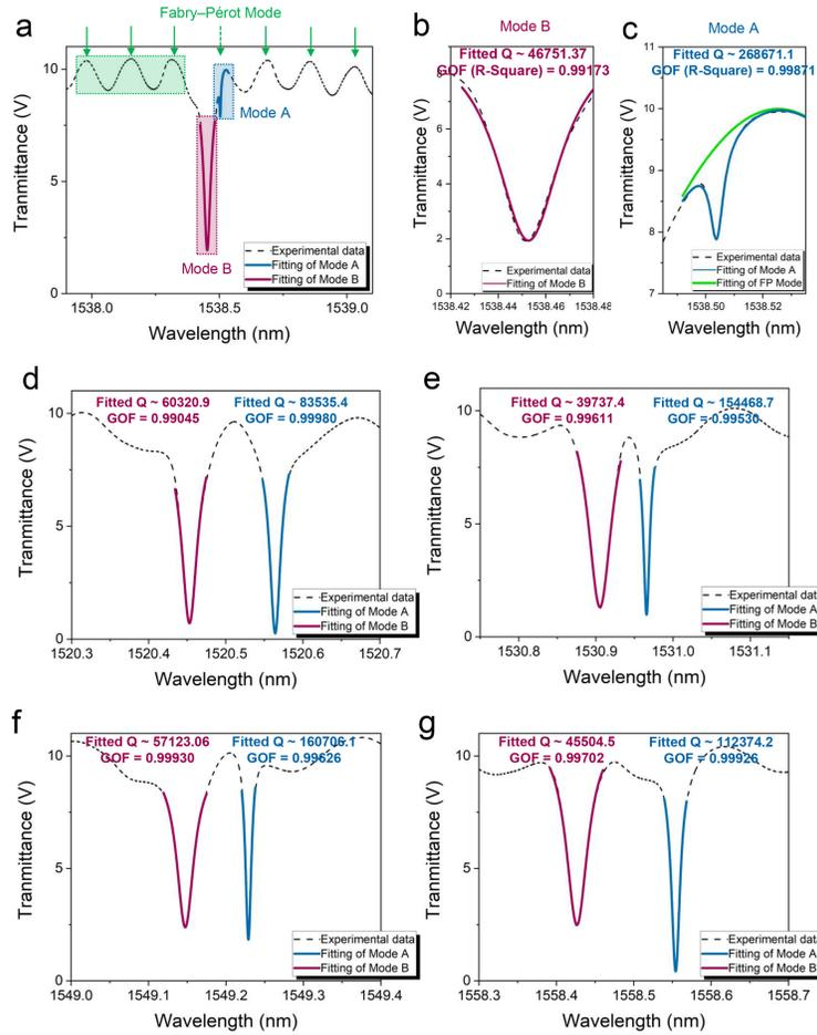
Fig. 7. Resonance fitting and  $Q$  factor extraction: (a) Transmission spectra near the quasi-BIC region, with green arrows indicating the Fabry-Pérot background caused by reflections at the bus waveguide edges. (b) and (c) Fitting results for Mode B and Mode A, respectively. (d) - (g) Fitting results for additional resonances.
