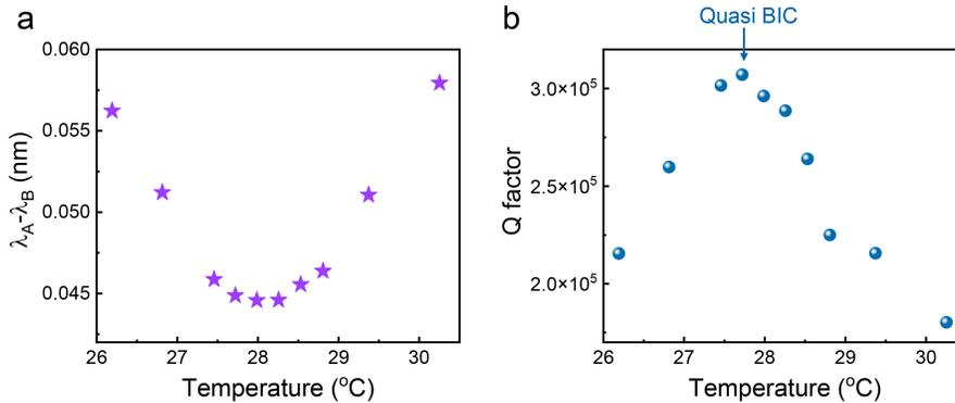
Fig. 5. Fine tune of the Friedrich-Wintgen quasi-BIC at Mode number 0. (a) Resonant wavelength difference and (b)  $Q$  factors of Mode A as a function of substrate temperature.
