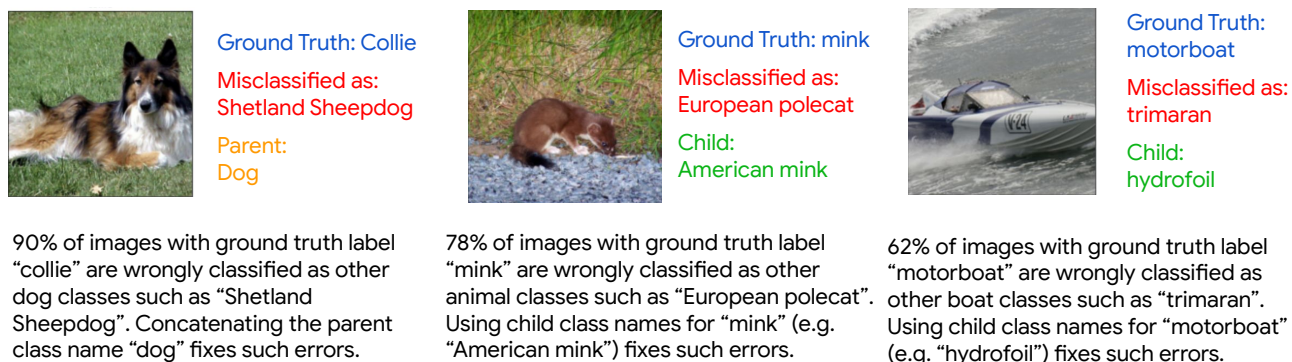
Figure 5. Qualitative visualization on typical failure modes for cases where our top-down and bottom-up prompt augmentation using the WordNet hierarchy method fixes the errors. In each case, the image is originally mis-classified but is correctly classified with our proposed method.
