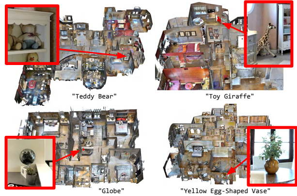
Figure 5. Open-vocabulary 3D Search. These images show the 3D point within a database of 3D house models that best matches a text query. The inset image shows a zoomed view of the match.
