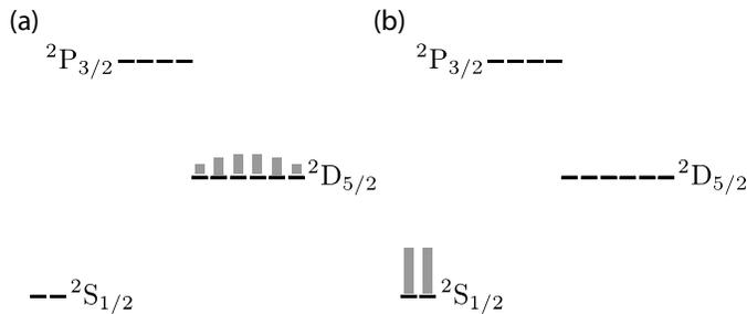
FIG. 1. Distribution of population before (a) and after (b) internal state cooling. The ion is prepared in a mixed state with a wide population distribution, corresponding to high von Neumann entropy. After thermal light is applied, the ion is left in the ground state with lower entropy.
