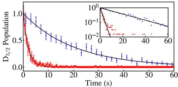
FIG. 3. Probability that the ion remains shelved after some time with (red) and without (blue) sunlight. Deshelve times longer than 60 seconds are included in the fit but removed from the plot for readability. Inset is a semilog plot of the same data.
