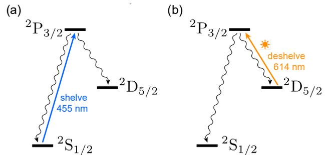
FIG. 2. A simplified schematic of the experimental sequence. (a) laser light is used to shelve the ion into the  $^2\text{D}_{5/2}$  manifold then extinguished, followed by (b) the sunlight pumping the ion back to the ground state. We measure the characteristic  $1/e$  time for step (b) by illuminating the ion continuously with laser Doppler cooling light while monitoring it for fluorescence.
