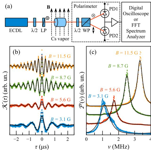
Figure 3. (a) Schematic of the experimental setup. (b) Spin-noise correlation functions, defined by Eq. (1), measured using digital oscilloscope (points) and their fitting by Eq. (2) (black curves). (c) The spin-noise power spectra measured for different magnetic fields using commercial FFT spectrum analyzer (points) and their fitting by Eq. (3) (black curves).
