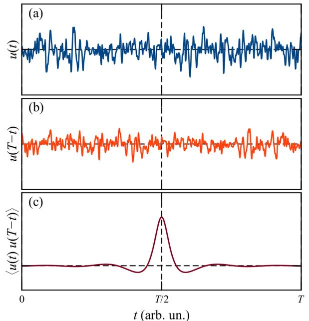
Figure 2. Getting correlation function via the time reversal. (a) A fragment of the detected noise signal. (b) The same fragment reversed in time. (c) Expected autocorrelation function of the signal, which can be obtained by multiplication and averaging over multiple realizations of noise traces.
