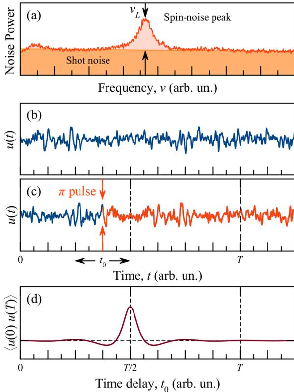
Figure 1. Typical frequency (a) and time (b) dependences of signals detected in spin noise spectroscopy. (c) Illustration to the *gedanken* experiment on observation of spin-echo effect in spin noise. The  $\pi$ -pulse is applied at  $t = t_0$ . (d) Expected dependence of cross-correlation of the noise signals at moments 0 and  $T$  as a function of  $t_0$ .
