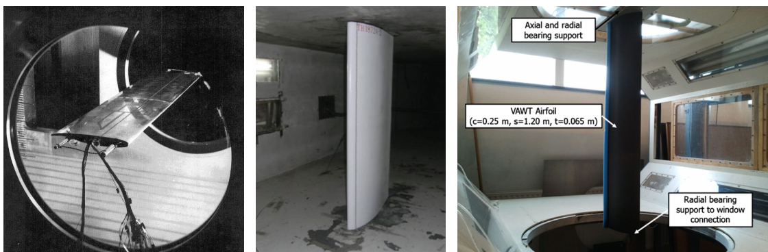
Fig. 3 “Infinite wing” test articles for wind tunnel experiments. From left to right: Refs. [31, 32, 33]
