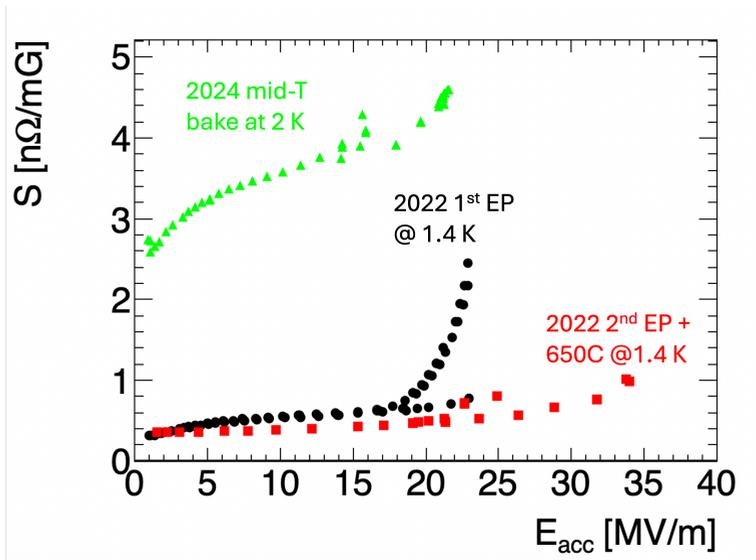
**Figure 4.** Estimated flux sensitivity as a function of accelerating gradient, assuming trapped magnetic field of 25 mG. The black circle points show data after 1st EP. The red squares show data after 2nd EP and annealing and annealing at 650 °C for 10 hours. The green triangles show the data after mid-T bake newly presented in this article.
