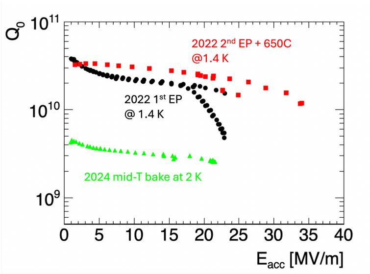
**Figure 3.** Comparison of quality factor as a function of accelerating gradient before and after mid-T bake. The black circle points show data after 1st EP. The red squares show data after 2nd EP and annealing and annealing at 650 °C for 10 hours. The green triangles show the data after mid-T bake newly presented in this article.
