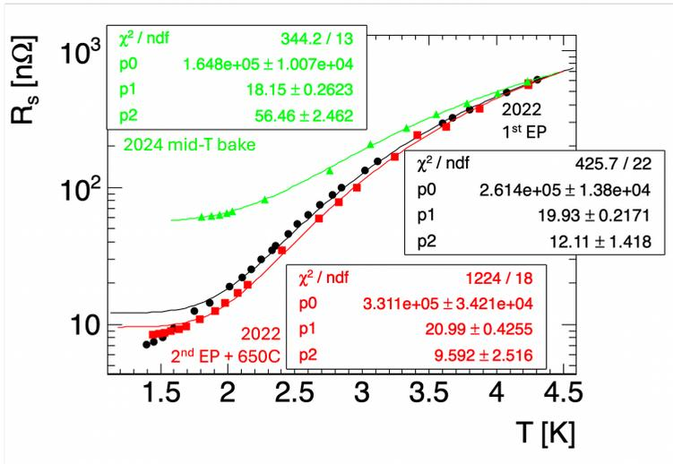
**Figure 2.** Comparison of surface resistance as a function of temperature before and after mid-T bake. The black circle points show data after 1st EP. The red squares show data after 2nd EP and annealing at  $650\text{ }^{\circ}\text{C}$  for 10 hours. The green triangles show the data after mid-T bake newly presented in this article. The solid lines are fitting curves.
