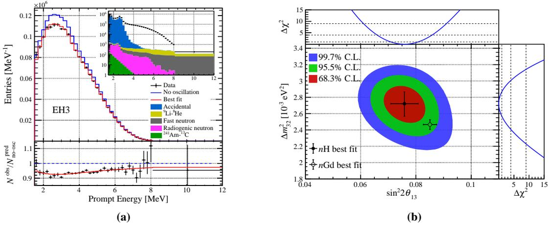
**Figure 2:** (a) Measured and best-fit spectrum distortion at EH3; (b) Confidence regions and best-fit points in the  $\Delta m_{32}^2$  vs.  $\sin^2 2\theta_{13}$  plane.
