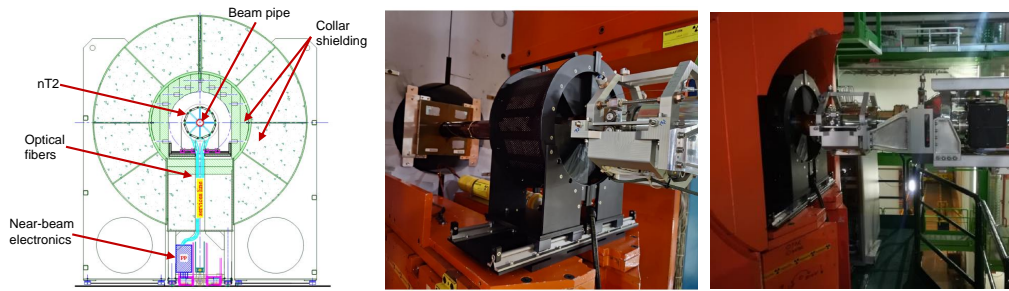
Figure 2: On the left, a drawing of the detector integrated in CMS. The beam pipe is perpendicular to the picture, in the center of the nT2 detector. On the center and right, two pictures taken during the installation training with a mock-up.
