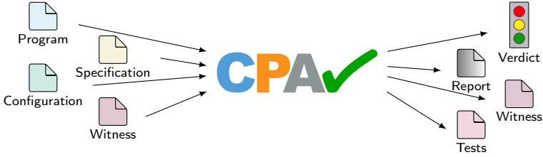
Fig. 1: Inputs and outputs of CPAchecker when it is used as a verifier , witness validator, or test-case generator
