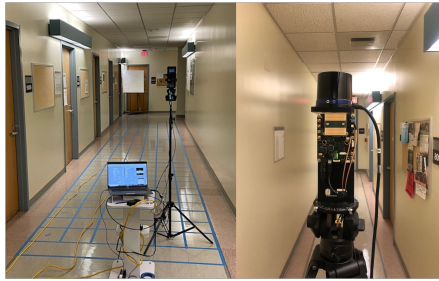
Fig. 2. Left: View of the L-shaped corridor featuring 102 grid points for RSS measurements, the receiver, and the flat foam board. Right: image of the collocated mm-wave transmitter and LiDAR at the end of the corridor.
