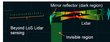
Fig. 3. LiDAR tracking of a user (1.8 m tall) in an L-shaped corridor using a mirror reflector. Mirror assisted LiDAR enables NLoS localization with centimeter level accuracy.
