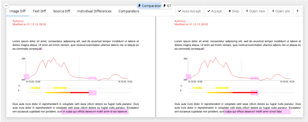
Fig. 16. A view showing visual differences between two PDF documents (differences are highlighted in magenta).
