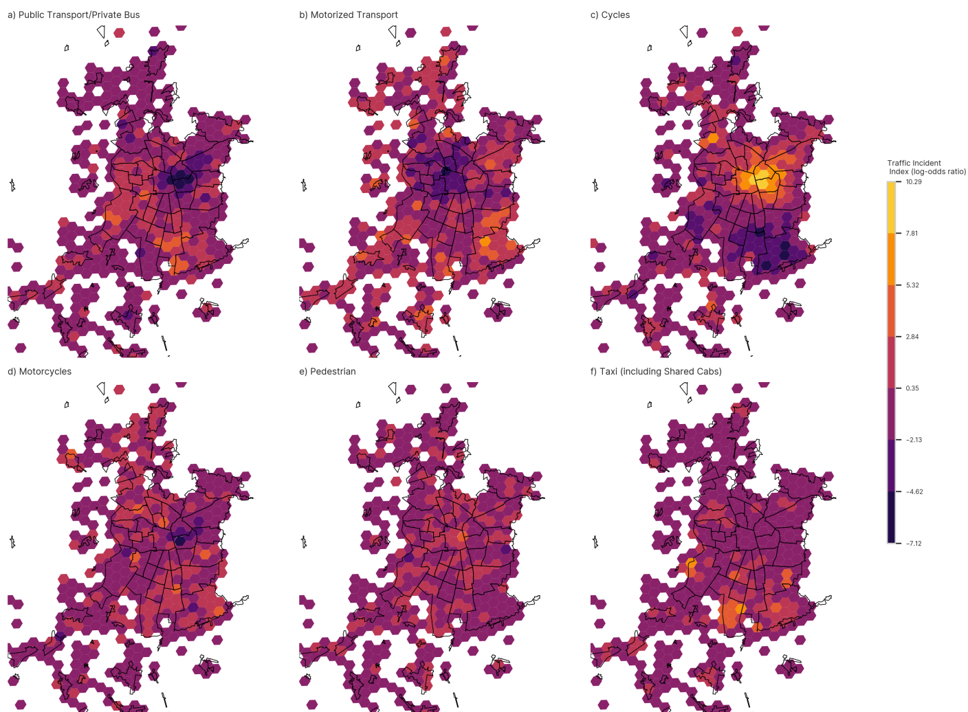
Figure 7. Spatial associations with mode of transportation in each incident with cells from the H3 grid system. The association is defined as a log-odds ratio with an uninformative Dirichlet prior (Monroe et al., 2008). Each mode of transportation has its own map: a) Public Transportation and Private Buses; b) Motorized Transport (private cars and other vehicles with four wheels); c) Cycles (including bikes and scooters); d) Motorcycles; e) Pedestrian; and f) Taxi, including shared cabs, which are used predominantly in the south of the city. Positive log-odds ratios, depicted in shades of orange, signify areas where incidents in the respective mode are more prevalent than expected. Conversely, negative ratios, depicted in shades of purple, indicate fewer incidents than anticipated.
