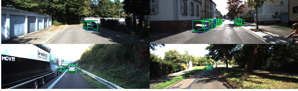
Fig. 5 Qualitative examples on the KITTI validation set. We provide four images. In the images, the green boxes represent ground truth, and the blue boxes represent predictions from MonoMM.
