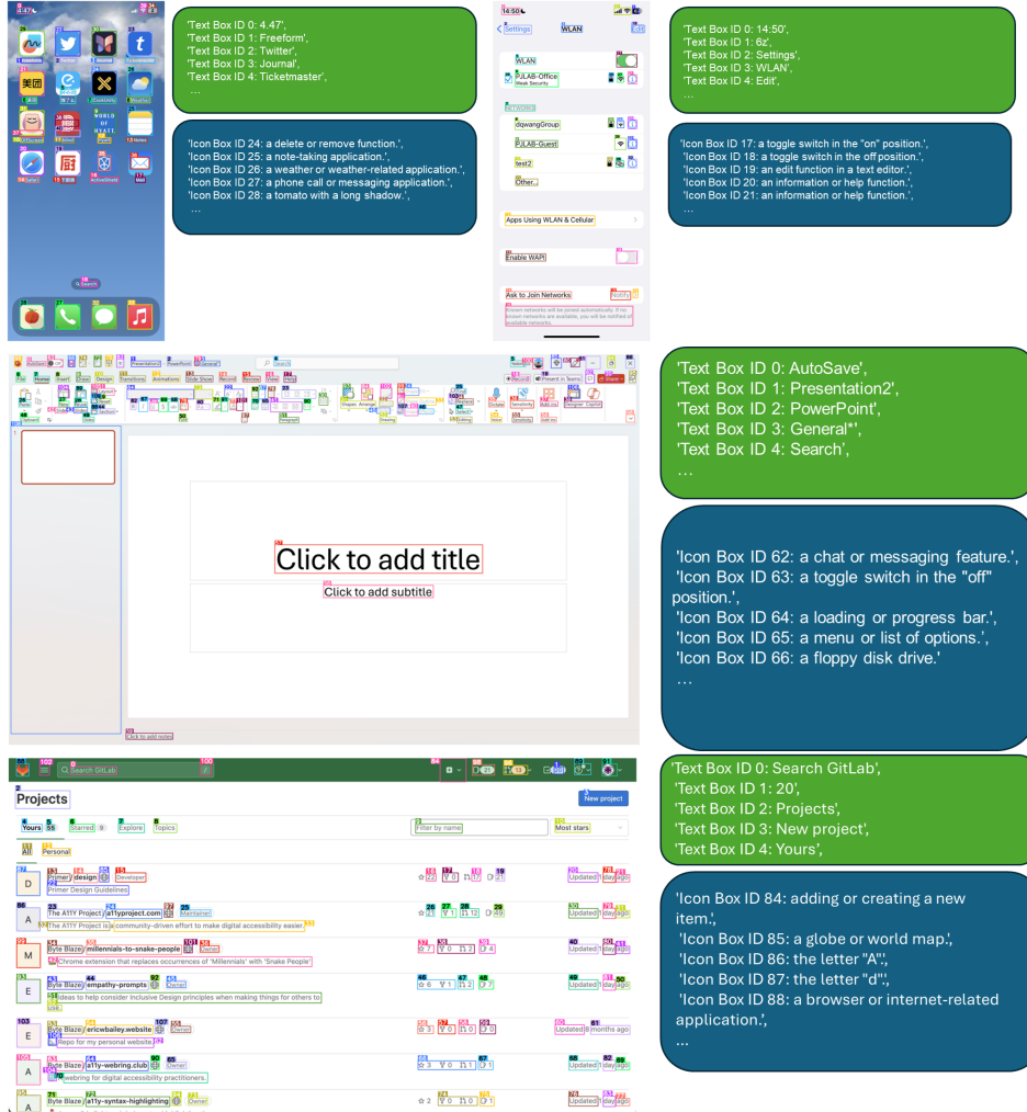
Figure 1: Examples of parsed screenshot image and local semantics by OMNIPARSER. The inputs to OmniParse are user task and UI screenshot, from which it will produce: 1) parsed screenshot image with bounding boxes and numeric IDs overlaid, and 2) local semantics contains both text extracted and icon description.
