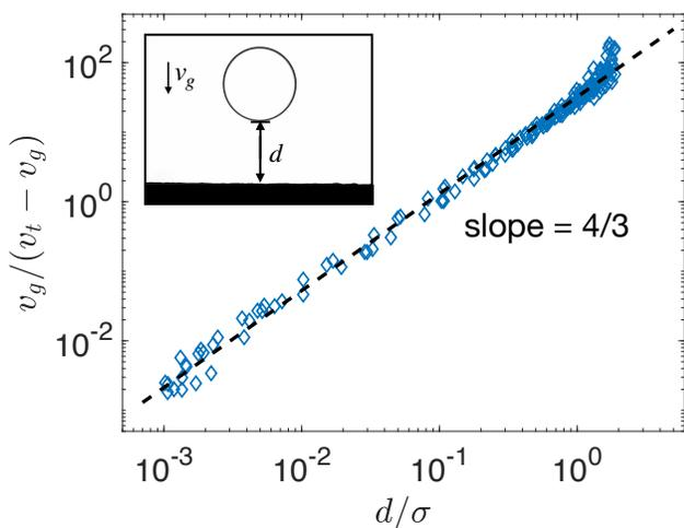
FIG. 10. The ratio  $\nu_g/(\nu_t - \nu_g)$  plotted versus distance  $d/\sigma$  from the chamber wall for the experiments. The droplet has diameter  $\sigma = 0.98$  mm, tilt angle  $\theta = 5^\circ$ , and terminal velocity far away from the wall,  $\nu_t = 0.65$  mm/s. An image from the experiment is shown in the inset. The dashed line has slope  $4/3$ .
