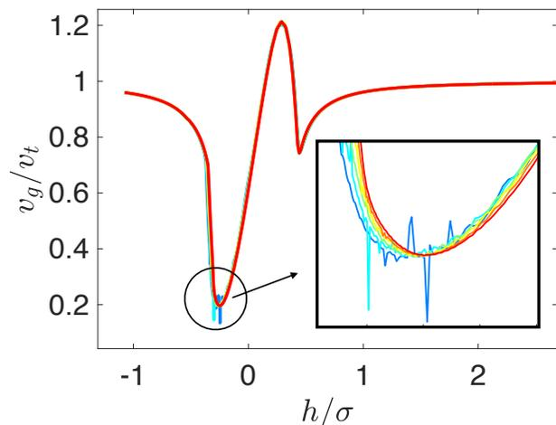
FIG. 11. Droplet center of mass speed  $\nu_g/\nu_t$  plotted as a function of distance  $h/\sigma$  from the orifice for DP simulations of a droplet flowing through a narrow channel with  $w = 0.7\sigma$ ,  $\Gamma = 1.08$ , and  $N_v = 32, 64, 128, 256, 512,$  and  $1024$ . The inset is a close-up of  $\nu_g/\nu_t$  near the first minimum in the speed at  $h/\sigma \approx -0.25$  to highlight the results for varying  $N_v$ , from 32 (blue) to 1024 (red).
