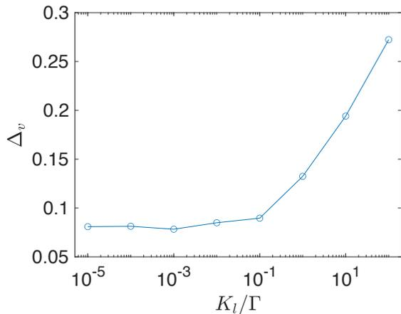
FIG. 12. Root-mean-square deviation in the droplet speed  $\Delta_v$  between the DP simulations and experiments for a droplet flowing through a narrow orifice with width  $w/\sigma = 0.9$  plotted as a function of  $K_l/\Gamma$ .  $\Delta_v \sim 0.08$  reaches a plateau for  $K_l/\Gamma < 10^{-2}$ .
