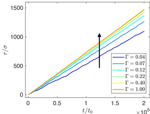
FIG. 14. Droplet displacement  $r$  in the flow direction  $r/\sigma$  plotted as a function of time  $t/t_0$  as the droplet traverses an obstacle array with  $w_{\text{ob}}/\sigma = 1.1$  and  $\sigma_{\text{ob}}/\sigma = 0.3$ . The arrow indicates increasing  $\Gamma$  from 0.04 (blue) to 1 (red).
