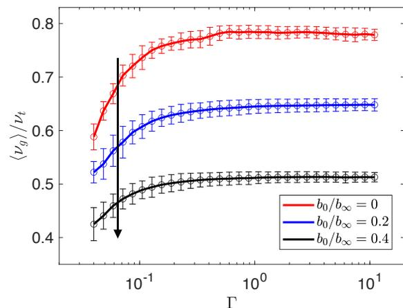
FIG. 15. Average speed of the center mass of the droplet in the flow direction  $\langle \nu_g \rangle$  normalized by the terminal velocity  $\nu_t$  plotted as a function of the dimensionless line tension  $\Gamma$  for obstacle arrays with  $w_{\text{ob}}/\sigma = 1.0$ . All other parameters are the same as those used in Fig. 8 (a), except we vary the near-wall drag coefficient:  $b_0/b_\infty = 0$  (red), 0.2 (blue), and 0.4 (black). The arrow indicates increasing  $b_0/b_\infty$ .
