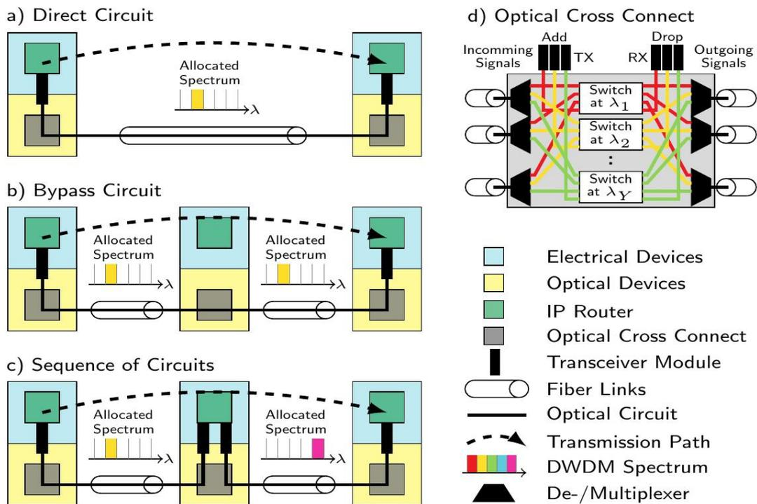
**Fig. 2.** a–c) Various ways of realizing transmission paths in wide-area networks with optical DWDM layer and d) architecture of a OXC as introduced in Witt et al. (2023).
