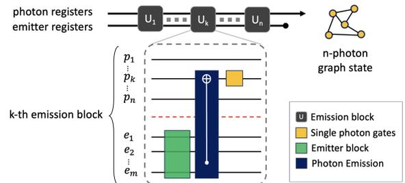
FIG. 1. Schematic of the circuit used for the sequential generation of photonic graph states. The main components are (i) single qubit gates on photons (yellow), (ii) emitter blocks representing arbitrary operations on the set of emitter qubits between emission events (green), and (iii) emission events (blue) corresponding to a two-qubit emitter-photon gate.
