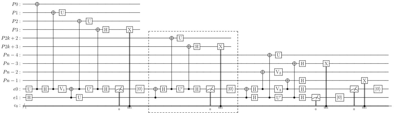
FIG. S3. The circuit to generate the best alternative graph in the orbit of an RGS with  $n = 2m + 8$  qubits. The elementary circuit block in the middle is repeated for  $1 \leq k \leq m$  while the rest of the circuit is fixed. For odd  $m$ :  $V_1 = X$ ,  $V_2 = U$ , and  $V_3 = U'$ , and for even  $m$ :  $V_1 = I$ ,  $V_2 = V_3 = H$ .  $U$  and  $U'$  are Clifford unitaries  $HPHPX$  and  $HPHP$  respectively.
