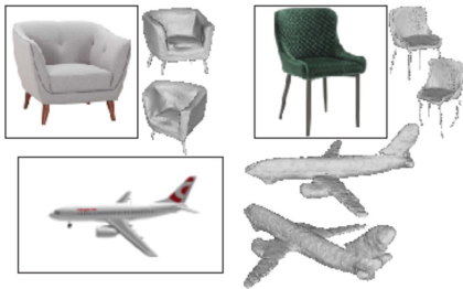
Figure 6: 3D shape from real images. Our results (right) produced from real images (left) While our results are not perfect, they provide reasonable approximation of the shown shape.
