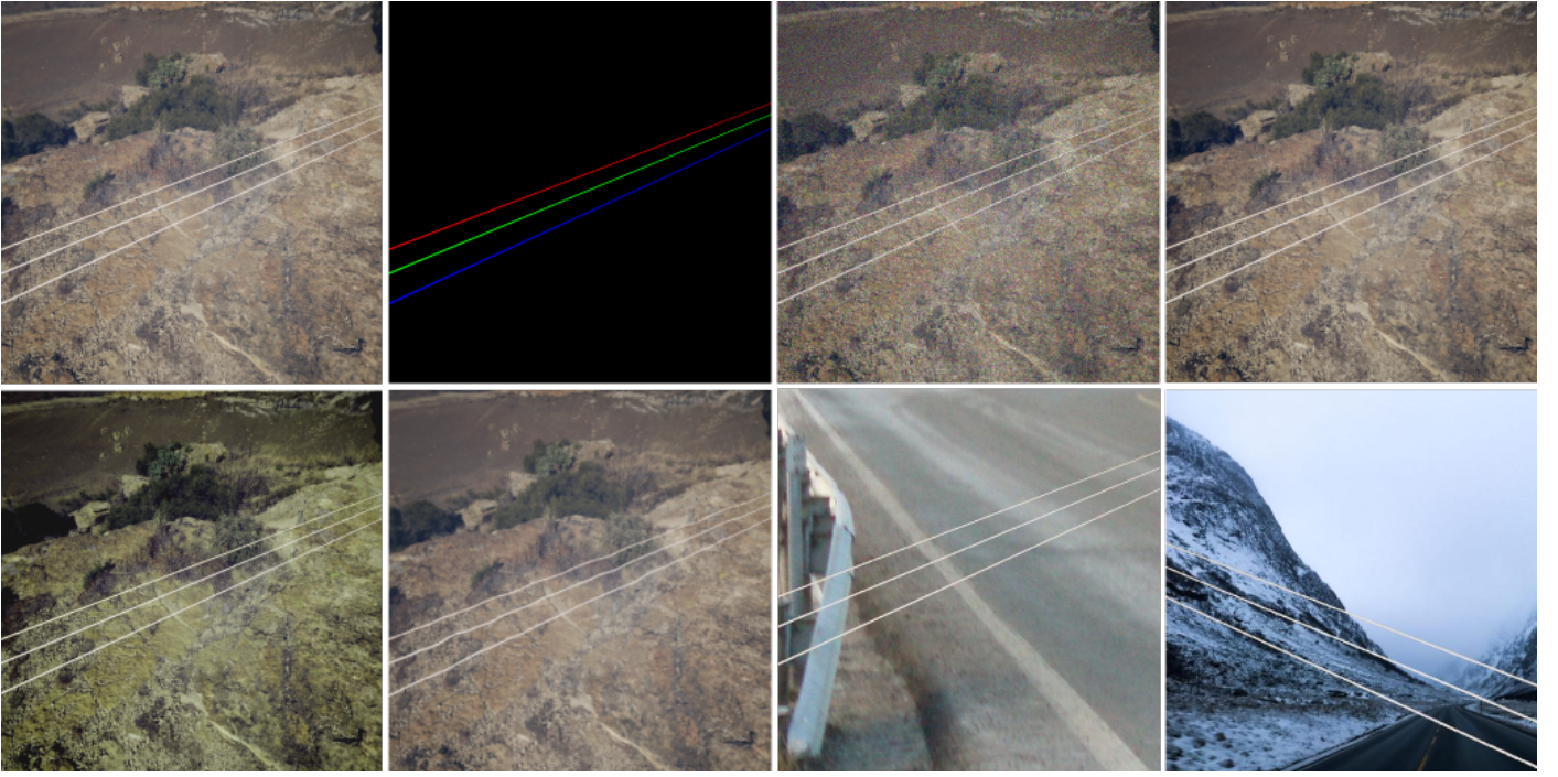
Fig. 1: Sample augmented images (from left to right): original image; pixel-level annotation, image with Gaussian-distributed additive noise; Gaussian blurred image; color manipulated image; elastic transformed image, image with new background, cropped and flipped image with new background.
