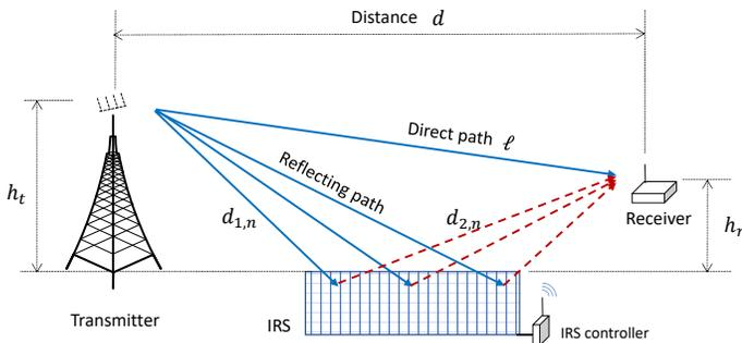
Fig. 6: Two-way channel model for IRS-assisted wireless communications.
