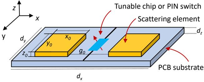
Fig. 4: Schematic of the unit cell for IRS, e.g., [46]. The basic topology and dimension parameters ( $d_x$ ,  $d_y$ ,  $d_z$ ,  $x_0$ ,  $y_0$ ,  $z_0$ ,  $g_0$ ) can be selected for operations in different frequency ranges. A tunable chip (e.g., diode and varactor) is incorporated to provide a variable impedance in a continuous way.
