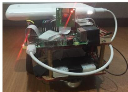
Figure 3. Image of autonomous vehicle prototype
