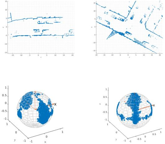
Fig. 2. Example from the KITTI dataset Geiger et al. (2013). Figures show two urban scenes pointcloud data and associated surface normals on a unit sphere. As seen, as the vehicle moves, the surface normals are also moving on the unit sphere which indicates the rotation between consecutive frames.
