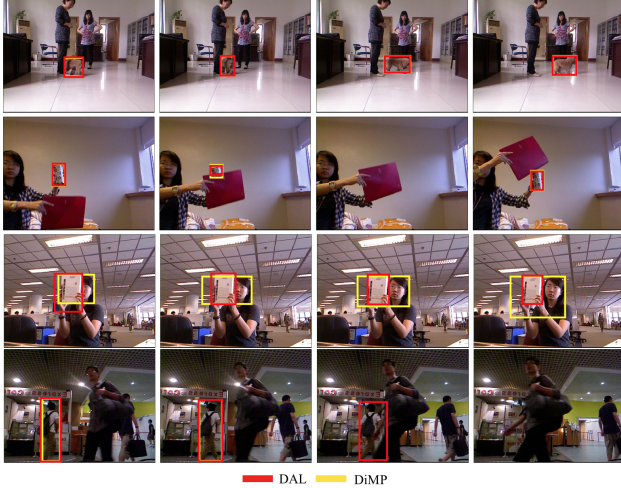
Figure 3. Qualitative comparison of DAL and DiMP. Both trackers localizes the target and give precise bounding boxes (the first two rows). With depth-modulated DCF, our tracker shows better discriminative ability when strong distractor appears (human face in the third row). Compared to DiMP, with conservative long-term tracking design, our tracker reports target disappearance more accurately.
