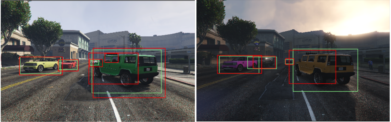
Figure 18: Failure images generated with Failure SCENIC Scenario 4 as shown in Figure 14 (b), with ground truth bounding boxes marked in green and prediction bounding boxes in red
