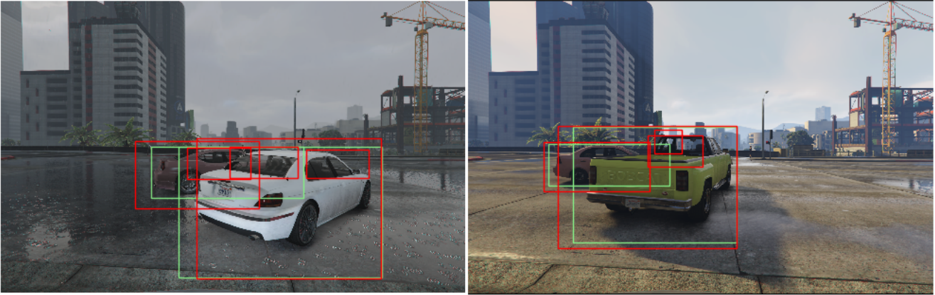
Figure 16: Failure images generated with Failure SCENIC Scenario 2 as shown in Figure 12 (b), with ground truth bounding boxes marked in green and prediction bounding boxes in red
