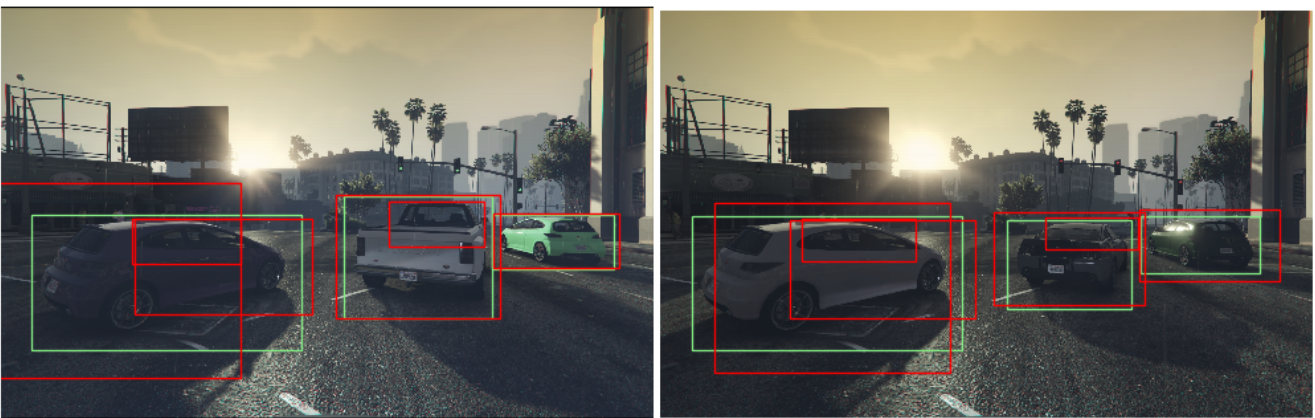
Figure 17: Failure images generated with Failure SCENIC Scenario 3 as shown in Figure 13 (b), with ground truth bounding boxes marked in green and prediction bounding boxes in red
