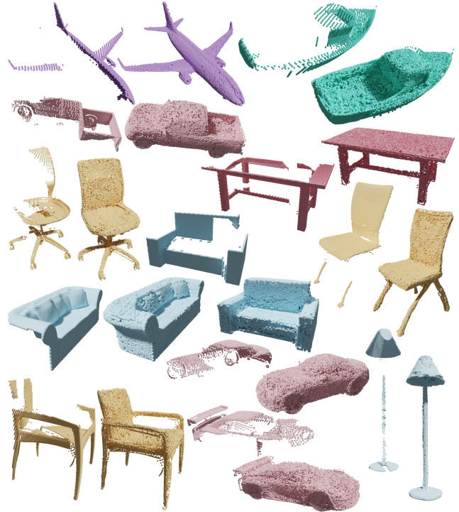
Figure 1: Our network predicts realistic structures from partial views and completes the point clouds evenly. Each pair (before and after completion) is visualized in the same color, with 32,768 points after completion.
