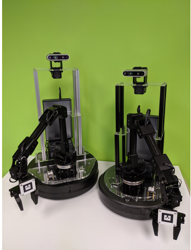
Figure 2: LoCoBot (left) and LoCoBot-Lite (right). Both robots have a 5 DOF arm mounted on top of a mobile base (Kobuki or Create2). Robots are equipped with a RGB-D camera mounted on a pan-tilt stand. Robots come with a battery pack and an on-board computer.
