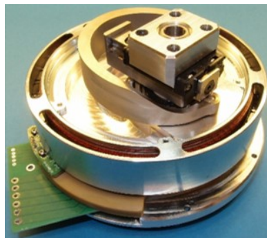
Figure 7: From top to bottom: photos of the prototype stiffness variation module (motor 2 with excentered disc), neutral position variation module (motor 1 with sliding pivot), and elastic module and output module assembled (motor 3 acting as damper, spring and linear guide).
