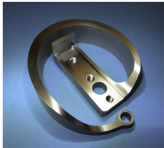
Figure 8: Finite elements simulation result and photo of the final spring design manufactured of titanium grade 5 (Ti6Al4V). The spring shape was iteratively optimized through finite element simulation to meet the desired stiffness of 60 N m/rad while making sure to not exceed the material fatigue strength and not touching surrounding parts at maximum deformation in either direction as the spring is asymmetric.
