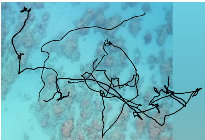
Fig. 6: The final paths swam by the Aqua robot covering over 1 km.
