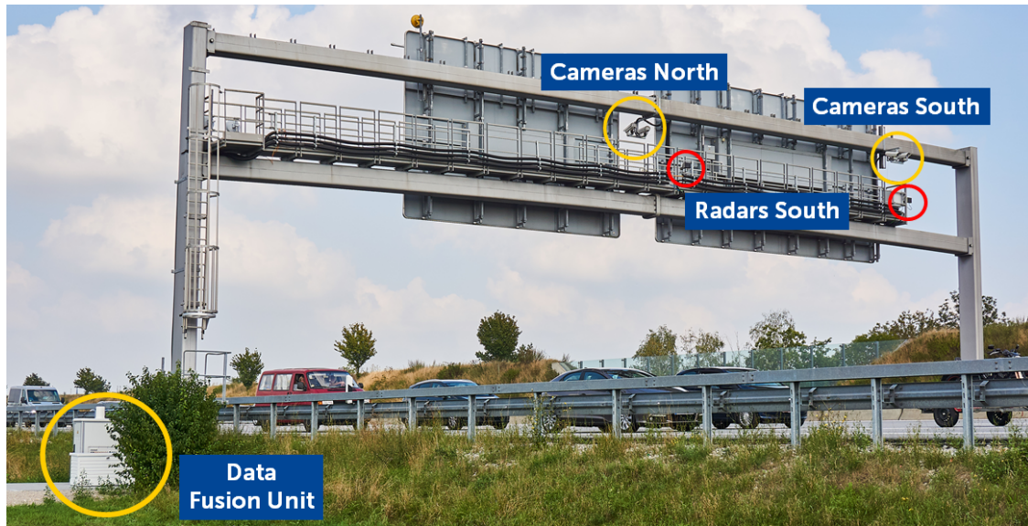
Figure 1: One of the Providentia measurement points on the A9 highway. The two radars directed towards the north are installed on the other side of the gantry bridge and are therefore not visible from this perspective.
