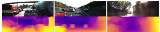
Figure 9: Example failure cases of our model can be due to unfamiliar objects, for example, the large tank truck and the bridge in the right image, or side vegetation (in the middle) and fence (right image).
